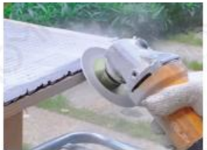
1.Grinding to make 45° chamfer
